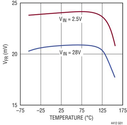
**V<sub>RTO</sub> vs Temperature and Supply Voltage**
