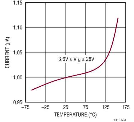
**I<sub>LEAK</sub> vs Temperature**
