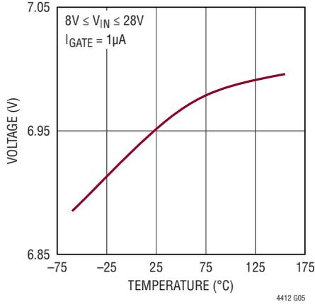
**V<sub>G(OFF)</sub> vs Temperature and I<sub>GATE</sub>**
